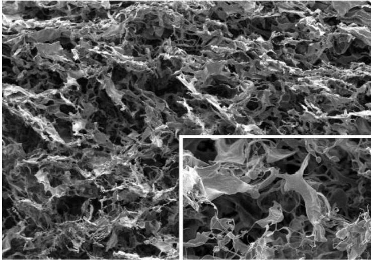
**Figure 1** Scanning electron micrograph of a collagen-chitosan blend cross-linked with 0.2% glutaraldehyde. Image is 100 $\times$  and inset is 500 $\times$  magnification.
